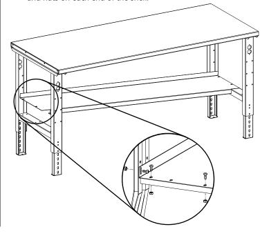
**5.** Attach the divider shelf to the cantilever upright frames. (See step 6 on how to attach). Using the help of an associate, place the upright frames with the divider shelf attached to the packing table. Use this as a template to mark the locations for the holes in the top. Remove the cantilever system off the top and unhook the divider shelf from the uprights.
