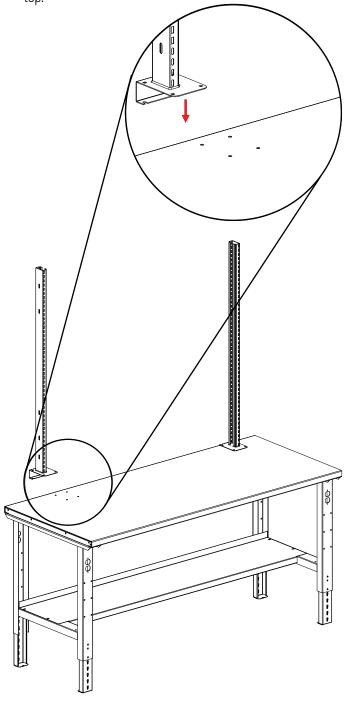
**6.** Attach the accessories (Ref. No.'s 5 - 11). Angle the piece so the back of the hooks are just above the holes on the upright frames. Slide the hooks into the holes and push down. Ensure both sides of each accessory is on the same level of holes on each upright.
