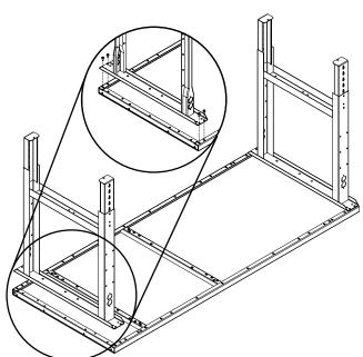
**3.** For assembly of a butcher block top, lay the top on a flat surface. Align the leg with the eight pre-drilled pilot holes. Attach with eight #14 x ¾" hex head slotted wood screws (Ref. No. 14). Repeat with second leg. Once finished,
