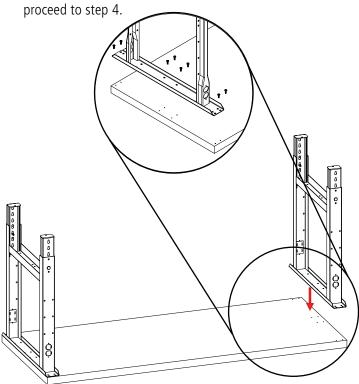
**4.** Turn workbench over. Place the lower shelf (Ref. No. 3) on the brace of each leg. Attach with three 1/4"-20 x 5/8" bolts and nuts on each end of the shelf.
